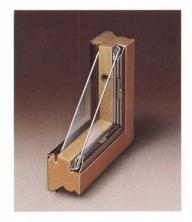
Pella's Double Glass Insulation System has a full 13/16" air space between panes. It actually outperforms welded insulating glass, yet costs less. Wood and vinyl separate the two panes of glass and function as a thermal barrier.
