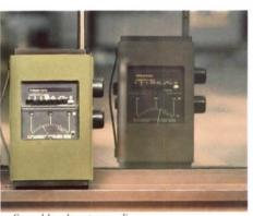
Sound-level meter readings: Interior 66 db, exterior 102 db.
