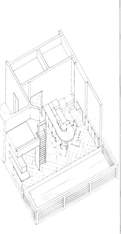
The original renovation of this 1850s brownstone established a one-bedroom apartment, but as the bedroom was only seven by eight feet—with an 11-foot ceiling, Rubin subdivided the space horizontally creating a sleeping loft above and a work space under. In the main space, he removed the massive marble mantle, rebuilt the fireplace wall and removed that portion of the bedroom wall that intersected the window wall.
