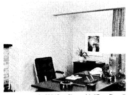
VINYL WALLCOVERING / Pictured is "Barn Door," a textured fabric-supported vinyl wallcovering for commercial applications. The design is on a bias, resulting in a chevron pattern; "Barn Door" is available in 10 color choices. The wallcovering meets Federal Specifications for heavy-duty vinyls, and is recommended for such heavy-traffic areas as hallways and lobbies. • Stauffer Chemical Co., South Plainfield N.I.
