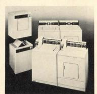
COIN-OP LAUNDRY EOUIPMENT / Heavy-duty commercial washers have energy-saving and security features. To cut water heating costs, a valve reduces the warm water ratio of "hot" water mixed with "cold" for both wash and rinse cycles; a "Power Miser" switch allows only cold water rinses. Money boxes are protected by high-security meter cases, and may be padlocked; the timer is also lockable. Sears, Roebuck and Co., Chicago, III.
