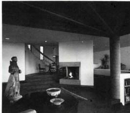
The principal interior finishes are oak strips for floors and gypsum board for walls and ceilings. Horizontal support members are either concrete or laminated wood beams.
