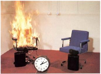
Ten and one-half minutes into this test the office chair constructed without VONAR is totally involved. The chair constructed with VONAR had ceased to burn when the paper fire went out (test details upon request).
