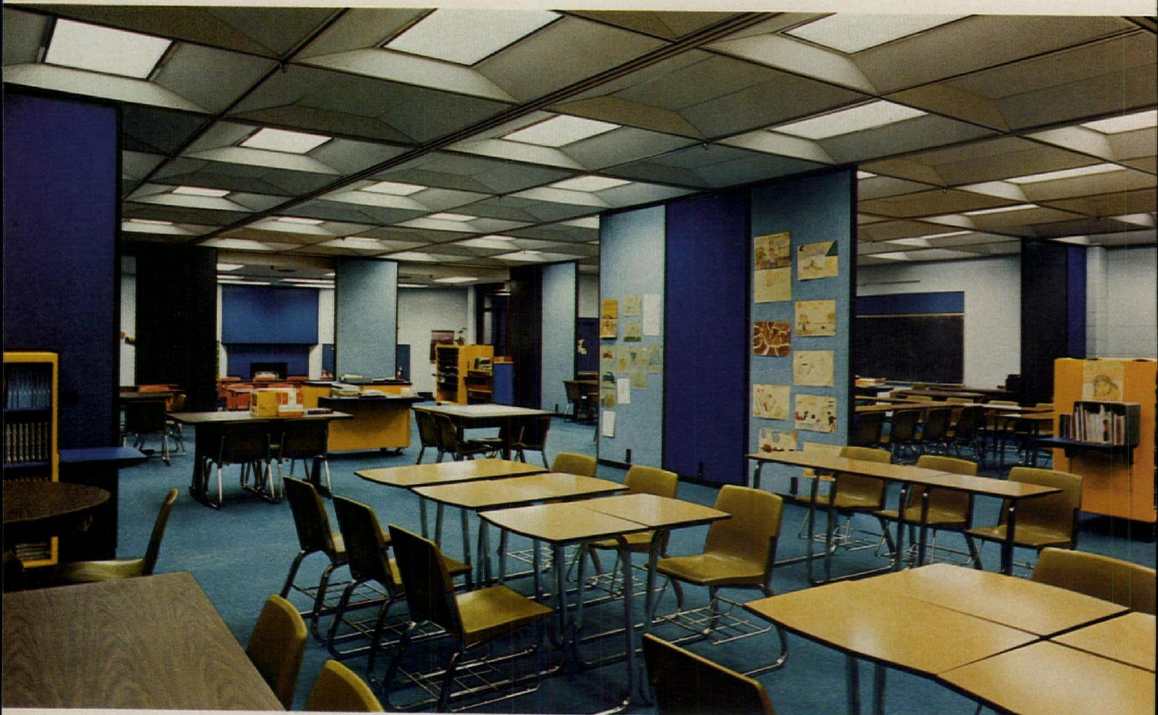
Open Plan arrangement at Jeffersontown School. Right angle tracks in ceiling permit open plan arrangement, above, or traditional classroom, as shown in top photo. Hartstern, Schnell, Campbell, Schadt - Louisville, architects.
