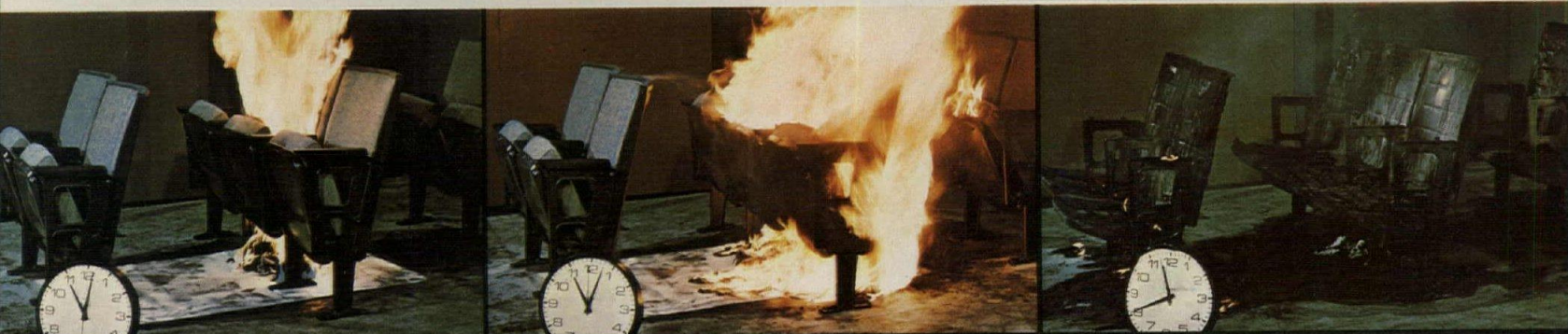
Major flames out. Time: 40 minutes, 00 seconds. Damage: All seven chairs involved.
