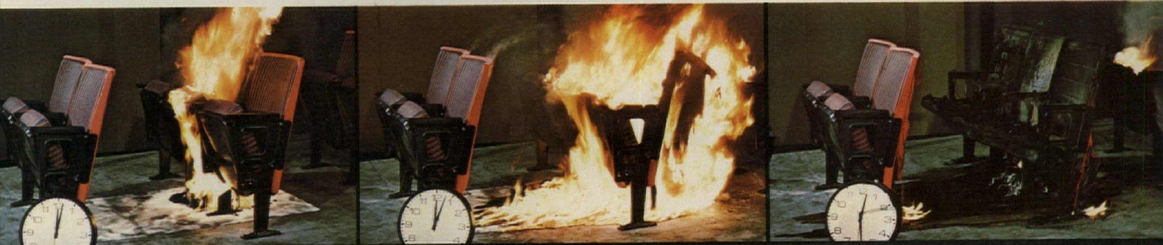
Time: 3 minutes, 00 seconds. Five chairs in two rows involved.
