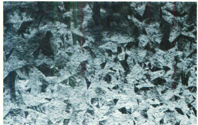
Galvanizing — the metallurgical bonding of zinc into steel — has proven its ability to protect rebar against rust before, during and after installation. This is recognized in the revision of General Services Administration guide specification PBS4-0344.01 as follows: When concrete cover on exterior surfaces is less than 1½ inches... reinforcing bars and mesh shall be zinc coated... in accordance with ASTM A-123.
