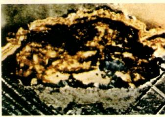
This magnification shows how rust expands as steel corrodes
