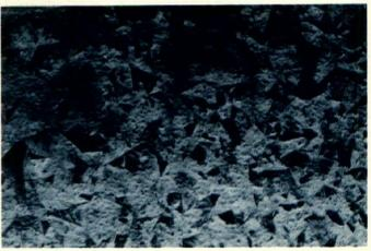
Galvanizing — the metallurgical bonding of zinc *into* steel — has proven its ability to protect rebar against rust before, during and after installation. This is recognized in the revision of General Services Administration guide specification PBS4-0344.01 as follows: When concrete cover on exterior surfaces is less than 1½ inches... reinforcing bars and mesh shall be zinc coated...in accordance with ASTM A-123.
