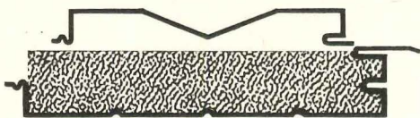
Varispan Panel System with 3" Glass Fiber Insulation. U-Value=0.111 btu
