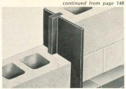
VINYL CONTROL JOINTS / Fillers are designed to fit standard sash blocks and provide a vertical joint for the relief of stress in concrete masonry walls. A range of sizes will accommodate 90 per cent of all masonry construction. ■ AA Wire Products Co., Chicago.
