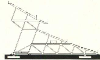
Movable stands have recently come into use to accomodate seating to the different configurations of baseball and football. So far, these stands have been set on railroad wheels or truck tires. Now air flotation systems have been proposed to reduce friction for movement. These illustrations show how the technique employed with Hovercraft vehicles (large fans and a flexible "skirt" to help contain air) could be used to lift a section of stands which then could easily be towed.
