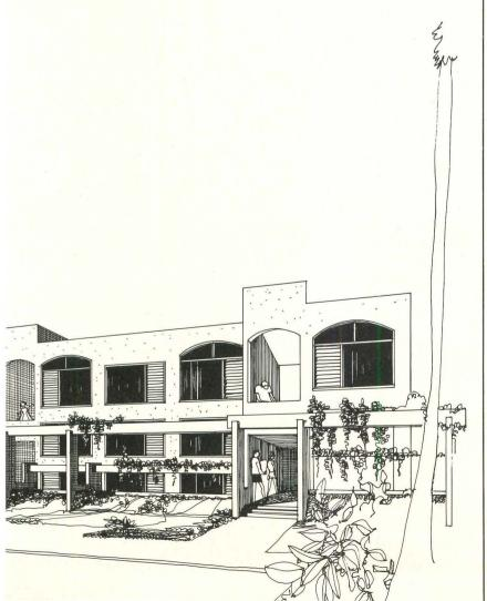
The building, a simple poured concrete and concrete-block structure, has been given variety and interest and brought into scale with the local village architecture by means of open stairways and broad trellises on the entrance side. The well-thought-out layout of the condominiums, shown in the plan below, permits the owner to conveniently and comfortably occupy all of his unit, or just the living and master bedroom, or only the second bedroom, if he chooses to rent out the remaining space.
