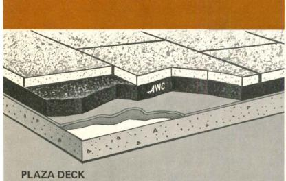
There are eight widely used All-weather Crete plaza systems. Not only does AWC provide the most effective available insulation, but it protects the water proofing membrane keeping it ductile and active for the life of the system.
