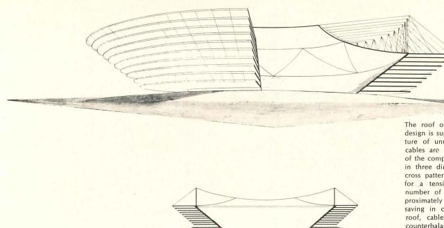
The roof of this proposed stadium design is supported by a cable structure of unusual configuration. The cables are stretched from one side of the compression ring to the other in three directions forming a crisscross pattern. This avoids the need for a tension ring, and thus the number of cable connectors is approximately halved—an appreciable saving in cost. The weight of the roof, cables and the live load is counterbalanced by the weight of parking ramps on the exterior.
