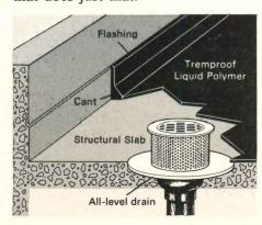
First, use a liquid waterproofing product that can be applied to the best-engineered concrete on the job site — the structural slab. Since the liquid adheres to the slab it will eliminate any lateral migration of water . . . . just in case it penetrates the seal.
