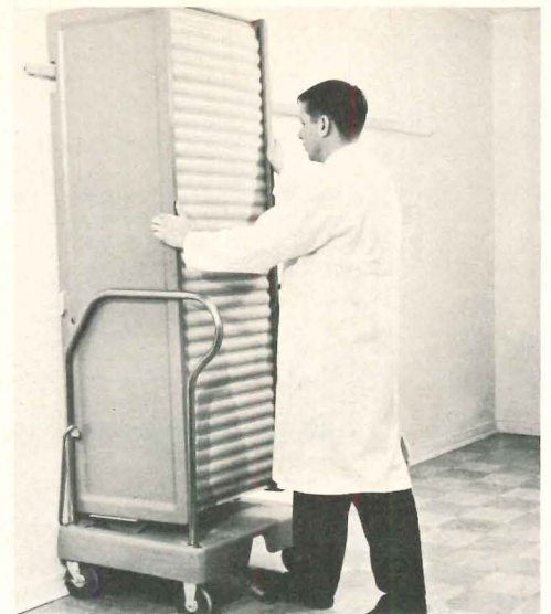
Carts for the closet-size containers can be hitched together in trains that track around corners and permit moving groups of storage spaces. Carts also have a pedal-operated lifter for installing and removing.
