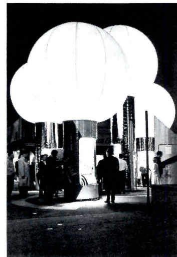
Prototype Pedestrian Information Center , Boston, Mass., Ashley/Myer/Smith, Inc., Cambridge, Mass., architects and planners, was a full-scale temporary working model to demonstrate and test a set of ideas for permanent centers. Eight brightly-colored kiosks topped by 12 foot translucent plastic balloons dispensed eight types of information.
