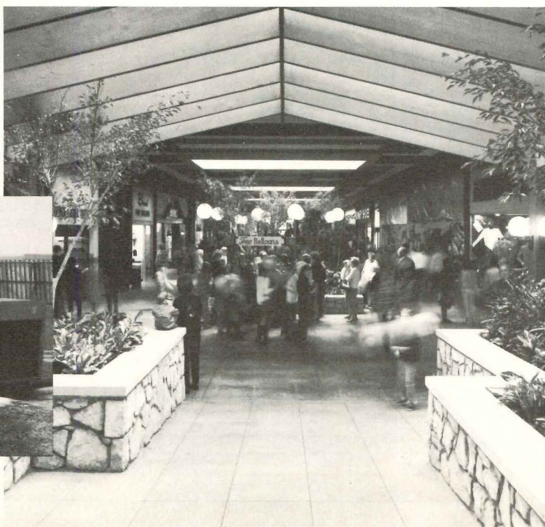
Phase II of The Mall was a major expansion, almost doubling the original 332,000 sq. ft. of the giant Louisville, Kentucky, shopping center. Shoppers' comfort in eighteen of the twenty stores, plus the mall, is assured by Lennox single-zone combination gas heating/electric cooling units. The twenty rooftop units, rated 3 to 22 tons, provide more than 200 tons cooling capacity. Architects: Katzman & Associates, New York City. Owner/developer: The Rouse Company, Columbia, Md. Heating/air conditioning contractor: Hussung Mechanical Contractor, Inc.
