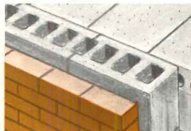
8 Cavity walls restrained in the vertical span.
