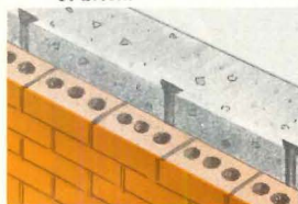
5 Flexible tying of masonry to concrete.
