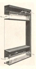
The Ventro Window is designed to provide ventilation, even in rainstorms with 110 mph wind conditions, without interfering with the design of the building. The window has no operating hardware, no projections inside or outside and no visual indication that the window is actually open. A simple baffled space provides the ventilation without leaks, drafts or bugs.
