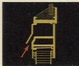
Kawneer's Pressure Equalization Slot keeps water out. Pressure within the window sections is equal to pressure outside the building. No pressure difference—no siphoning action—no leakage.
