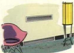
Concealed, floor-mounted arrangement
