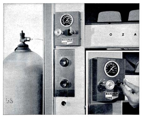
Ozalid<sup>®</sup> Anhydrous Ammonia System consists of control box mounted on machine and tubing to connect equipment with anhydrous ammonia cylinder, which may be remotely located. Developer handling becomes simply, "valve on, valve off."
