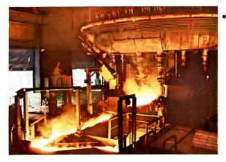
• Tapping molten iron from a blast furnace
