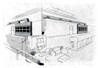
1. Weathermakers can be combined in many ways to fit various situations. Here, large units with short runs of ductwork handle a big manufacturing area, while another unit may handle the factory office space.
