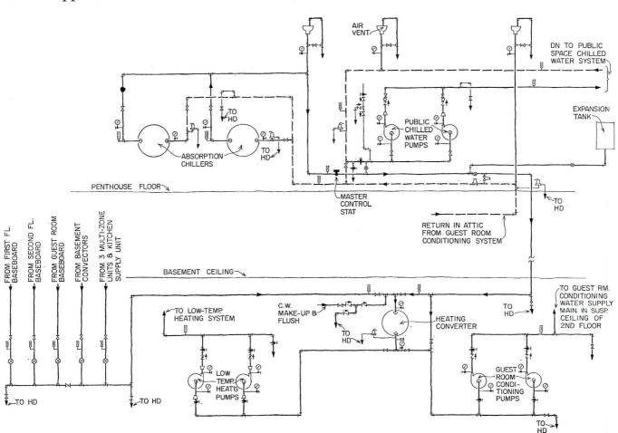
Piping diagram for heating and cooling water circuits in basement and penthouse at Water Tower Inn, Chicago (Hausner and Macsai, architects, William Goodman, consulting engineer; see Building Types Study, this issue) shows how a fairly simple system for fan coil cooling with baseboard heating and separate mechanical ventilation in guest rooms of a 15-story hotel-motel can be neatly integrated with other systems for public spaces
