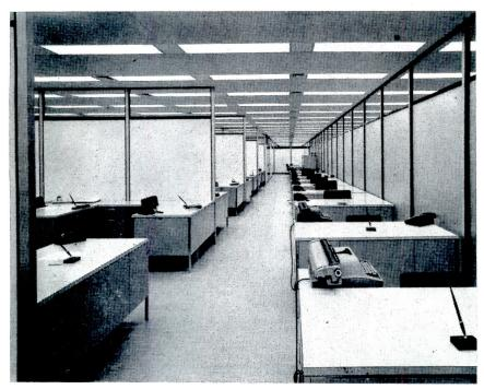
Depth of girders due to wide spans made the continuously luminous suspended ceiling, variants of which have been used successfully in other SOM jobs, impossible at Chase. Ceiling reflectors used here are not stock size. They were specially made at an increased width to reduce surface brightness and glare. Square units between lighting fixtures permit diffusers for return or supply air, or are blank. Partitions cross on the blank spaces
