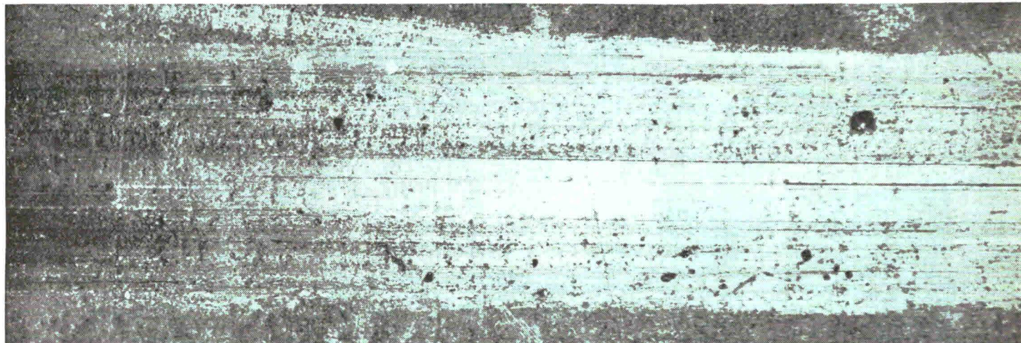
HERE YOU SEE THE LAPIDOLITH treated concrete after 500 strokes. Note that even under six magnifications the surface appears unbroken, with total wear being measured at only 0.0003 in. The equivalent of 1/3 of 1 mil! Particles of metal may be seen imbedded in surface of the concrete.
