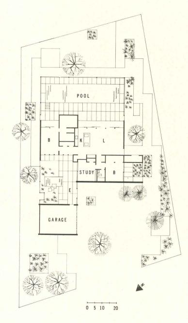
THE STRUCTURE: The house is built of a special concrete block, exposed inside and out and finished with silicone. The blocks are 8 by 16 in. and precisely stacked for neat appearance. Beams are spaced on a 6-ft module, which becomes a module for the interior spaces. The foundation is reinforced concrete, with all floors finished in terrazzo. The roof is surfaced with 4-ply tar and gravel. All wood is pressure treated. Insulation is foil-enclosed, 4-in. batt.
