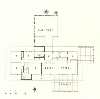
THE PLAN: A slight drop in the site is used to give a multi-level scheme, with ceiling heights varied to the size of the rooms. Entrance, bedrooms, and kitchen-dining areas are on one level, with a step down to the main living area. Below this is a sort of contemporary inglenook with a fireplace. The flue from the fireplace passes underneath the entry slab (5 ft above the floor of the lower living room) and rises through the utility room adjacent.
