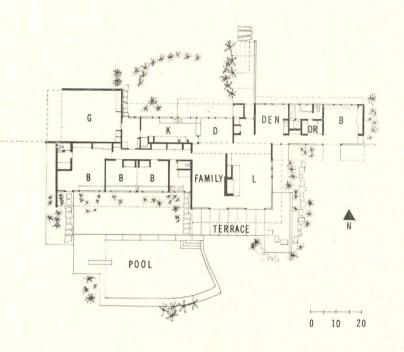
THE STRUCTURE: A post and beam frame of wood and steel permits considerable flexibility in the plan, and adds to the sense of openness and space. The exterior is finished with non-bearing walls of wood, stone and stucco. Floors are reinforced concrete slab. The roofing is composition. Window sash is aluminum.
