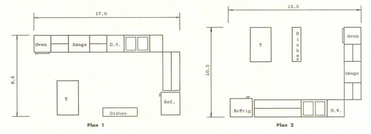
The most compact kitchen which meets all of the standards previously suggested is illustrated in *Plan 1*. The area of the plan is 161.5 sq ft. Some persons might object to the fact that the dining table would probably be on an inside wall. This objection is overcome in *Plan 2*, but here the sink is on the inside wall. This would seem to be a greater fault than that in Plan 1
