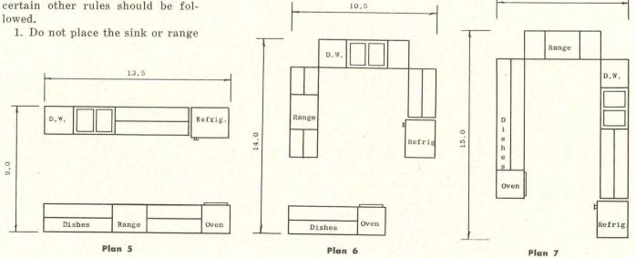
If the mix center is placed between sink and refrigerator, as in the preferred sequence, the corridor arrangement increases in size to 189 sq ft (Plan 5). Extra desk storage is in the kitchen proper. Plan 6 (252 sq ft) and Plan 7 (255 sq ft) require more space, but also result in larger dining areas
