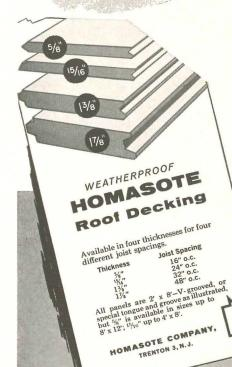
In one strong piece of weatherproof material, you have top structural strength, insulation, sound-deadening and an attractive finished ceiling. Application is simple and speedy. As evidence of Homasote's strength, note that the 1%''thickness spans 48", where other materials require 3" thickness.
