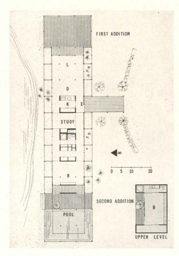
CONSTRUCTION: Due to a somewhat marshy site, the foundation was formed by a grid on 8-ft centers of drilled reinforced concrete shafts, 12in. diam. and 12-ft long. Wood 4 by 4 columns were erected on these bases. Floor and roof framing consists of two 2 by 8 beams on 8-ft centers, and 2 by 6 joists on 16-in. centers. Exterior walls are glass or asbestos-cement panels painted white. The roofing is built-up tar and gravel. Windows are all fixed 1/4-in. plate glass.
