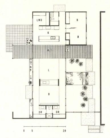
STRUCTURE: The Jared house is built on a lot which, when acquired, had an existing cut and resultant "shelf," which obviated the necessity for any further site work, though a retaining wall, enclosing the garden, was required. The foundation is concrete, the framing fir timber. To integrate visually the basic structure with the retaining wall, the beams are carried out to "reach out and grab it."
