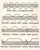
Interior and exterior sheets formed of: aluminum; galvanized, aluminized or stainless steel, and with all mill finishes and architectural colors.
