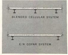
LESS FRAMING. Cofar reinforced concrete design permits wider spans, saves on structural framing costs, speeds up building completion and permits earlier occupancy by the owner.
