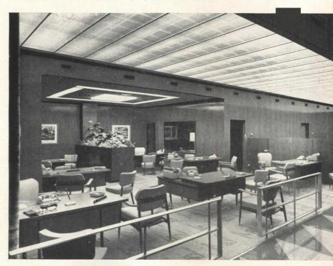
Even with Strato-Lux directly overhead, there are no bright spots, no reflections, in critical viewing areas. Acrylic plastic panels never discolor, can be slipped out one at a time and dipped in detergent for cleaning.
