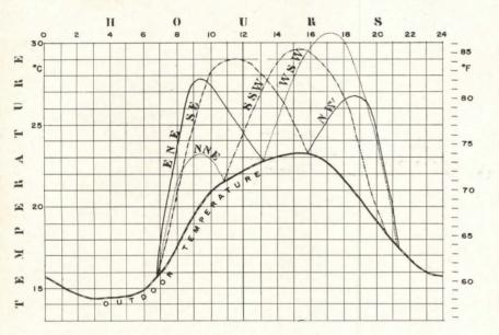
FIGURE 2b. Temperatures, determined by formula, which would exist inside rooms if no sun control devices were used. Indoor temperatures were calculated by adding the effect of sun radiation (Fig. 2a) to the outdoor temperature, assuming a 2-hr time lag. To plot this, 12.5 Btu per sq ft are assumed equal to a 1 F rise in temperature, based on studies by Prof. C. P. Yaglou of Harvard
