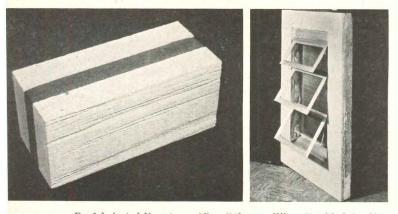
Prefabricated limestone: (1) a "thru-wall" unit with 3-in. limestone, 2-in. cellular glass, 3-in. waste stone; (2) window surround with 1-in. stone, 3-in. insulation and sprayed aggregate
