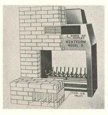
HEATFORM MODEL D is a fireplace unit serving two rooms, in which air chambers capture and circulate a large volume of the heat instead of losing it to the chimney. The unit has air heating chambers above and below the firebox, with connecting heating chambers leading from the lower to the upper heating chambers. It is shipped with a square end steel bar fuel grate made of <sup>3</sup>/<sub>4</sub>-in. bars for wood burning only. Superior Fireplace Co., 1708 East 15th St., Los Angeles 21.
