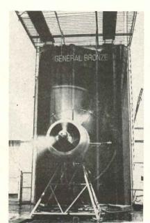
Propeller drives water from overhead pipes against building mock-up
