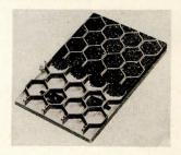
Hexteel safety floor armor can be used in new concrete floor installations or in conjunction with a mastic fill on existing concrete or new wood floors. It forms a continuous steel floor armor which is said to eliminate cracking, swelling, warping and shrinking and is designed to take the brunt of rolling loads. The exposed steel surface is 18.15 sq in. per sq ft of floor, and the weight of the Hexsteel is 1.7 psf. Klemp Metal Grating Corp., 6603 So. Melvina Ave., Chicago 38, Ill.
