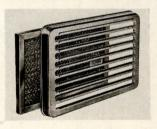
Electric ceiling ventilators with combination grille and filter unit screen out grease and dust. Trade-Wind Model 2501, which delivers 425 cfm, and Model 1501, with 300 cfm, are optionally equipped with the new filter. The design of the combination unit includes a special grille about 1 in. deep into which the cleanable metal filter is fitted. Trade-Wind Motorfans, Inc., 7755 Paramount Blvd., Rivera, Calif.
