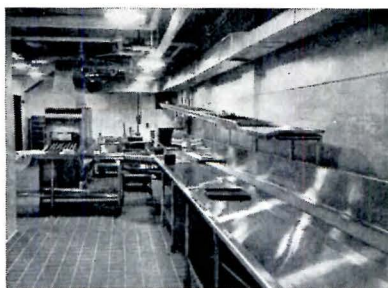
Conveyor system carries dishes away for washing after pre-wash at Duke University
