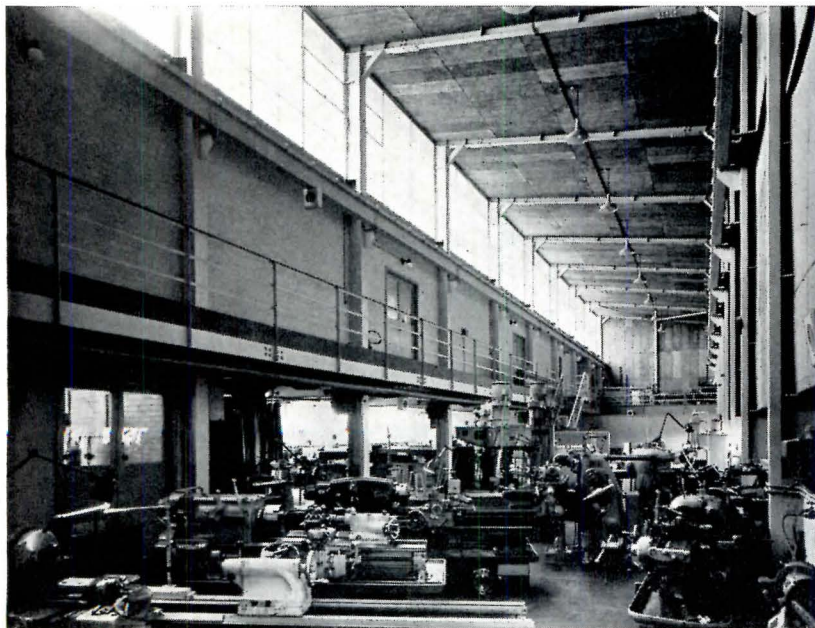
Physics School Workshop (left), upper level; walls are 3-in. insulation blocks against asbestos cement sheets; right, High Tension Laboratory
