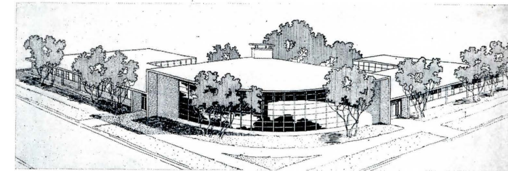
Top: men's dormitory, Colorado A & M — four three-story dormitory wings with central two-story lounge-dining unit; capacity 400, cost $1.5 million, area per occupant 248 sq ft; architect, James M. Hunter. Above: women's dormitory, Upper Iowa University — two one-story L-shaped wings joining central high-ceilinged lounge; capacity 54, cost $238,000, area per occupant 265 sq ft; architect, William A. Lockard. Below: men's dormitory, Tufts College (Mass.) — three- and four-story, includes dining facilities; capacity 280, cost $1,065,000, area per occupant 239 sq ft; architect, Arland A. Dirlam
