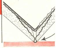
Here's why Super-Ex corners are stro last longer: note greater depth of pl adjacent to bead area... spring fit v adapts easily to any specified dep plaster ground — whether it be  $\frac{3}{4}$ ", or  $\frac{1}{2}$ "... and solid metal that pr corner at point of greatest strain.
