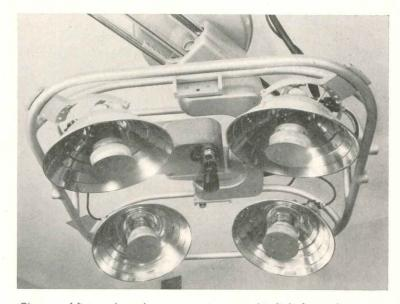
Closeup of fixture shows how camera is mounted in light frame. Lamps are special color-balanced units, designed to permit best possible color
