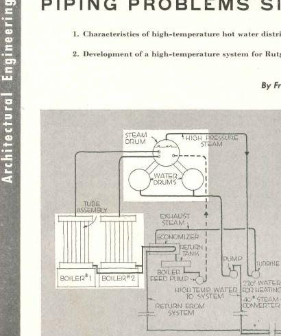
Schematic diagram of the hightemperature hot water system for Rutgers University. High-temperature water flows from drums to steam or medium-temperature hot water convertors in each building. High-pressure steam operates the turbine-driven circulating pumps. The return water is preheated by the exhaust steam
