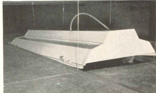
The fixture rests on the grid rails. End baffles lock the compression feature into place. No hangers or suspension straps.
