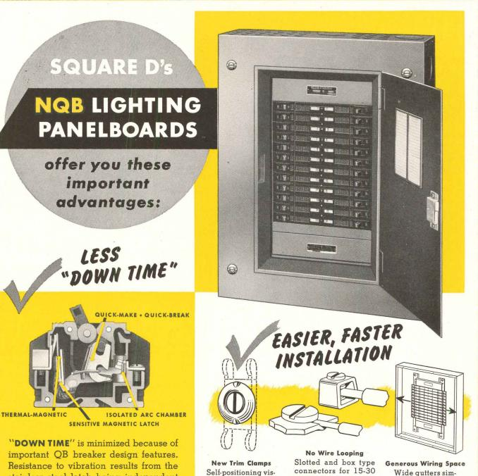
stainless steel latch being independent of the trip element. Thermal (coilless) magnetic trip affords 2-way protection. Thermal element holds harmless momentary overloads but trips if excessive current continues. Magnetic element responds instantly to heavy overloads or shorts. Simple reset operation restores service quickly when the breaker trips. New Trim Clamps Self-positioning visual indication of clamp position speeds installation.
