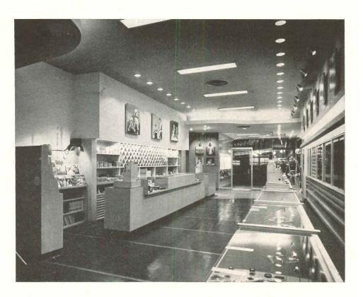
Directional lighting through incandescent spots over counter, also gooseneck reflectors over picture display on right wall and over book display case
