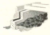
External vapor generated by uncovered earth in crawl spaces may be greater than all other sources combined.
