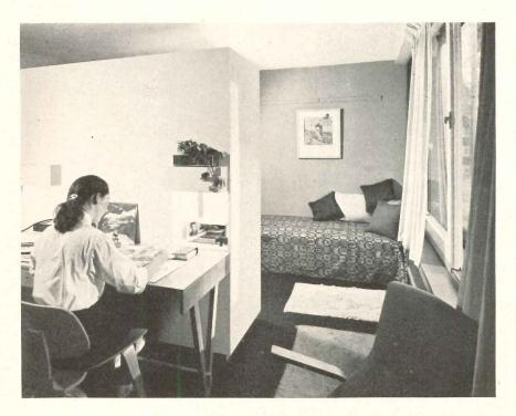
Typical double bedroom is divided into sleeping space and study space by head-high cabinet partition. On one side are aligned two study desks, each with inset lighted panel. Other side of this same fixture lights dressing table in sleeping portion
