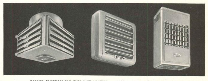
**CARRIER PROPELLER-FAN TYPE UNIT HEATERS.** Four-way Directed-flo vertical model 46S gives quick heat from higher ceilings. Discharges in four directions, at any angle, in any quantity. Steam or hot water. 7 sizes: 82,000 to 500,000 Btu's. Horizontal model 46U directs warmed air from heights of 15 to 18 feet. Attractive, quiet, rugged. Single-row Aerofin heating coil with
