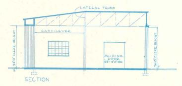
A N OLD IDEA IN HANGARS for large planes appears here in new form. The large plan shows its simplest form, a sort of minimum hangar for the occasional large plane. Diagrams at the right show how the same general idea might be used in various combinations, with shop areas included, for different types of planes. All of these assume that the whole plane need not be in the hangar. Canvas drops are used in many.
