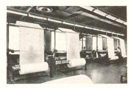
\$1500 Saved Here. This unique inspection method uses 24 forty-watt Sylvania fluorescent tubes and a luminous panel. Mill engineers estimate this Sylvania-designed unit provides a saving of \$1500 per year.
