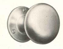
YALE knobs and roses, #D35 and G222 A knob within a knob, the #D35 has a bronze finish spun over an inner shell of steel. Result -beauty with strength and resistance to indentation. The perfect companion, rose #G222 is finished in bronze as well.
