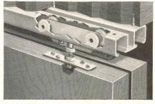
SERIES 600—A new double track designed for  $1\frac{3}{6}$ " by-passing wardrobe and closet doors. Has newly designed adjustable hanger providing convenient means of aligning door to side [amb. Allows 1/2" vertical adjustment.
