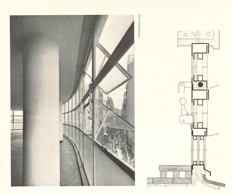
Above, left: typical office floor. Above right: section through window wall; bottom pane is fixed obscured glass. Below: baseboard detail showing use as electrical duct
