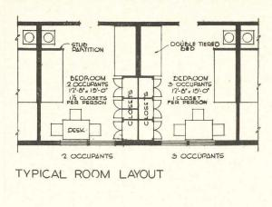
Each typical room has three closets, full ceiling height, with built-in drawers and upper storage compartments. For two-man occupancy, center closet is cut in half
