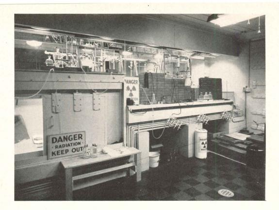
In this semi-hot laboratory at Brookhaven National Laboratory, two types of shielding are provided. The sliding lead door provides easy access in setting up an experiment. A barrier of lead bricks can be adjusted to suit the experiment. Mirrors along the back wall enable technicians to observe and operate equipment at a safe distance
