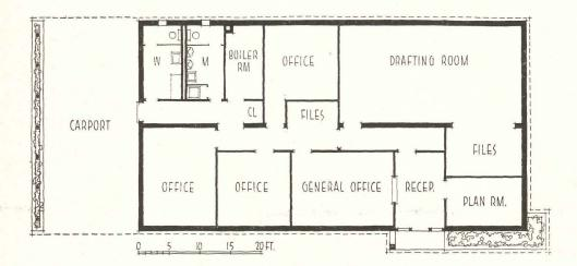
The omission of windows in this compact, trim office building serves both to reduce costs and lessen distraction from outside noise, and also permits flexibility in the placement of furniture along walls. Openings in toilets on plan are exhaust louvers
