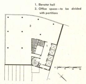
Setbacks of the building follow city regulations. The structure is of reinforced concrete, with brick used in dark areas of section shown left. Numbers indicate floor use: 1. shops; 2. bank; 3. offices. The three top floors follow plan shown above. Utilities are dispersed on each of lower floors to aid in office rearrangement
