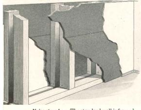
Noise stops here. The standard wall is framed with  $2 \ge 4$ 's on a  $2'' \ge 4''$  plate. Secondary wall is framed with  $2 \ge 4$ 's turned flatwise on a  $2'' \ge 2''$  plate with a half-inch space between plates. Both walls are lathed with sounddeadening INSULITE LOK-JOINT LATH.
