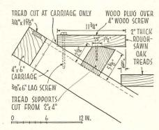
Stair hall was disengaged from other elements so easy stair proportions would not be cramped. As wood adjusts to atmospheric moisture, lag screws are taken up to eliminate squeaking treads. Cantilevered nosings add to stair's resiliency. Rail is 1-in. round iron; balustrade, wire rope. Garage, below, has vertical lift doors; old architectural documents are stored on upper level
