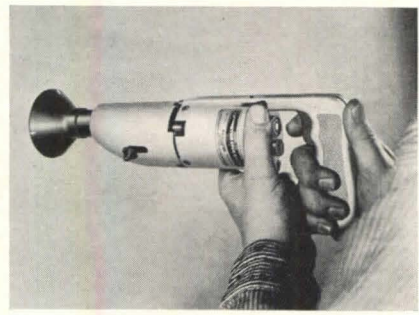
Lightweight stud driver fastens powder propelled studs into steel, concrete
