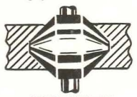
SIDE VIEW OF CONCEALED BEARING SUPPORT Rounded surface maintains valuable streamlining.
