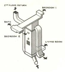
Preassemblies used: left above, shop-fabricated copper plumbing ''tree''; framing is designed around it to minimize cutting. Left below, prefab stair; above, warm air heater and complete prefab ducts; chimney is also prefab. Below, heater in kitchen closet
