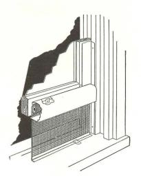
Plastic screen automatically rolls into housing as window is lowered, appears in place as window is raised
