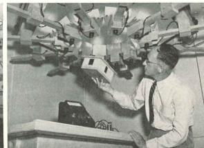
Scientists of the Commonwealth Experimental Building Station, Sydney, Australia, demonstrate artificial 'sun'' (left) and 'sky'' (right). When full-scale 'sky'' is built, models will be placed in center of inverted bowl, 24 ft across. Continuous fluorescent tube will replace the adjustable lights used for development
