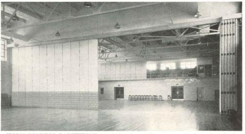
• HORN FOLDING PARTITIONS are designed to utilize space and offer a long lasting, efficient operation. Manufactured in a new, modern factory according to specifications a Horn Folding Partition is factory installed to insure maximum operating life. There is a Horn Folding Partition for every problem!
