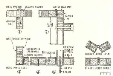
paperboard with alternate layers in opposing directions. Facing is waterproof plywood; edging strips, wood; adhesive, phenolic resin. Roof-joint taping has been improved for later models
