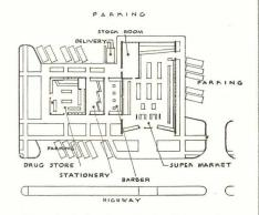
Plan includes two Luria Standard Buildings, Supermarket, 60 feet wide and 100 feet long with 16-foot eave height. Shops, 40 feet wide and 80 feet long, with an eave height of 12 feet.
