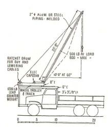
More preassemblies: left above, trussed rafters and gable ends erected by special truck-mounted aluminum crane designed by the architects; right, large windows (optional) with shop-fabricated rough frames, site-applied casings
