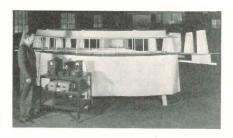
Ultrasonic sound tests on scale model predict acoustics of proposed structure
