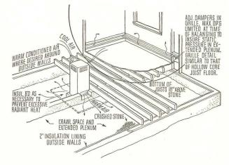
Warm air from the bottom of the furnace fills the crawl space and heats the floor in this ductless system. Grilles with adjustable dampers around outside walls admit air to the room
