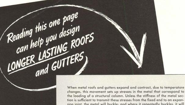
sion joint, the metal will buckle; and where it repeatedly buckles, it will soon crack. Thus, one basic factor in non-ferrous\* sheet metal construction usually
