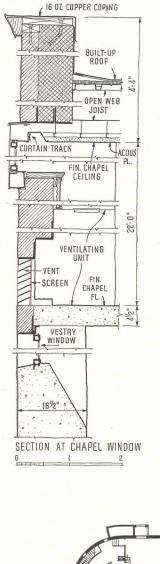
Plans were worked out to give all parts of building direct access from entrance court and yet to segregate various activities. Semi-circular bima in chapel and enclosed choir posed unusual problems in acoustics. Curved wall surface was broken up into panels for sound control (as in radio studio design) and vertical louvers were set in on either side of Arc to permit choir to be heard (details at right, photos opposite). Chapel seats 560
