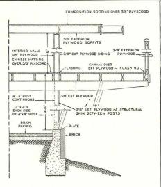
Typical section shows Exterior-type plywood employed as structural skin between  $4'' \times 4''$  posts, 6' o.c. Interior walls, 1/4'' plywood, were resin-sealed, given coat of grey paint, wiped to desired grain show-through, and waxed. Interior and exterior joints covered with narrow battens.
