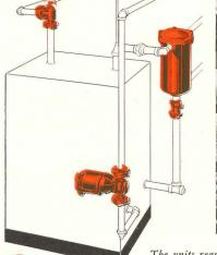
The units required for B & G Hydro-Flo Heating are few and simple. They can be applied to any bot water heating boiler, whether oil, gas or stoker fired.
