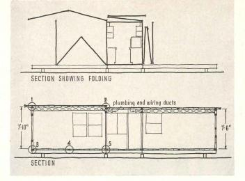
Diagrammatic section shows how The Acorn House is unfolded after placement on its light steel subframe. Typical joint details at right also show standard panel construction, corrugated
