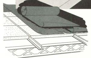
SIMPLE FAST CONSTRUCTION Kaylo Roof Tile are laid on subpurlins or structural steel members or nailed to wood joists. End joints are grouted. Roofing material is applied on tile. No special skills or tools are required, and one man easily handles the 23-lb. tile.
