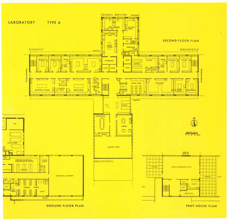
the various elements to be found in a laboratory building of this type. The basic requirements, such as the type of laboratory work to be done, the allotment of space to each department and local site conditions, will vary so much that it would not be possible to develop a plan that would be suitable to all situations. It will be found that the departments and their component elements as shown in these plans will exceed minimum requirements of some states and be somewhat below those of others.
