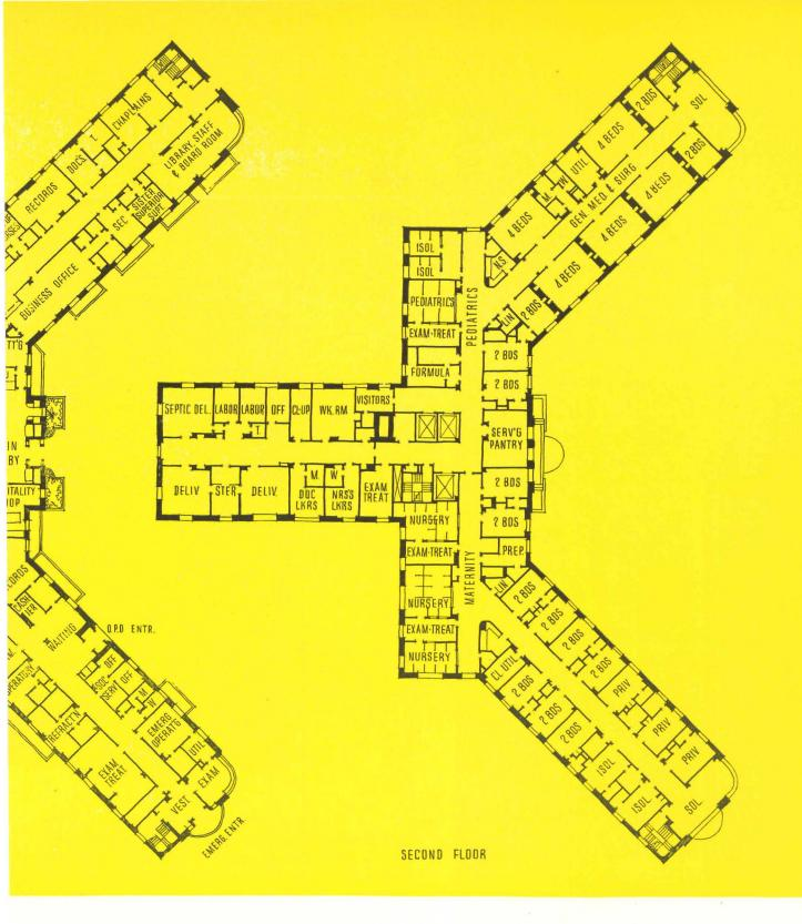
that the service elevator is so arranged as to have access to the basement service corridors and completely segregated from the passenger elevators, so that easy access can be had to the housekeeper's suite, laundry, and linen exchange, as well as to the female locker rooms. It will also be noted that the main kitchen serves directly into the hospital service elevator for distribution of food to the bed floors by means of heated food cart circulation.
