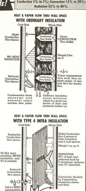
HEAT FLOW thru space of NON-INSULATED WALL:
