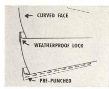
CURVED SURFACE, installed under tension, makes rigid, sound-resistant, insulating siding with weatherproof joints, beautiful shadow lines without wrinkles. Easy to apply. Low construction costs!
