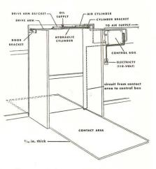
Door control uses no motors or gears
