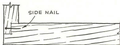
SIDE NAIL LESS EXPENSIVE DRAWER CONSTRUCTION (HAS LATERAL WEAKNESS)
