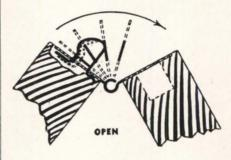
Tempered spring transforms butt-hinge into one that is reported self-latching
