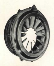
Exclusive with York, a gradual acting multi-radial vaned control, constructed of accurately machined non-ferrous materials. Ring and pinion gear movement insures smooth vane opening and closing—multiple vanes give precise adjustment of refrigerant flow down to minimum capacities . . . impart a flow pre-rotation. Result—inherent stability of operation over the widest capacity ranges.
