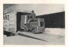
Trucks and trailers loaded without steel plates or bridge ramps by application of a hydraulic loading ramp, the Leva-Dock
