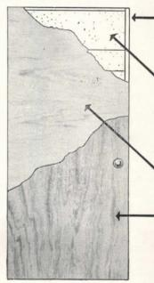
**EDGE BANDS** are thoroughly kiln dried hardwood, built up of two pieces of  $\frac{3}{4}''$  stock, securely glued together to provide greater dimensional stability.
