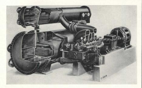
The use of "volutes" in the design of the centrifugal compressor which forms a part of the Worthington Centrifugal Refrigeration System provides greater efficiency because the smooth, obstruction-free gas passages reduce friction and turbulence loss.
