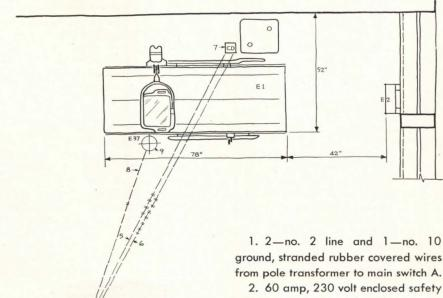
switch A fused for 60 amp; locate 4 ft. 6 in. above floor in position shown or above junction box B, if desired.
