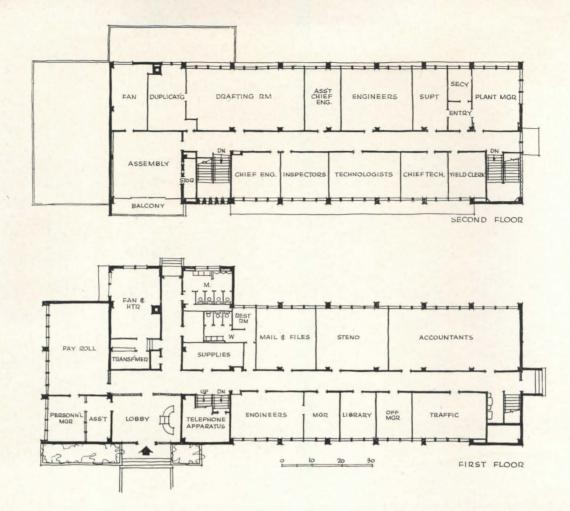
Both buildings (this one and the Martinez office building) were designed on a 4-ft. module — columns on 16-ft. centers, windows and fluorescent fixtures at 4 ft., air supply outlets 8 ft. on center from plenum chamber over corridors. Steel universal forms 2 by 3 ft. dictated the height of this concrete building at 12 ft. floor to floor. Overhangs are a continuation of the floor slabs
