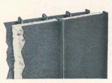
INSULATED STEEL WALL (FIELD CONSTRUCTED)
