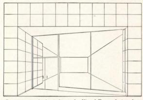
1. Here are the basic lines of a Visual Front, designed so that passersby see the entire store interior through a clear glass front. But glass can do more—it can direct attention to the front and the interior by effective use of *Vitrolite* facing on solid areas.
