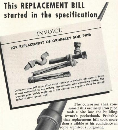
Stop that replacement cost now. Specify Acid Proof Duriron for Chemical Laboratory drain lines . . . and for any other corrosive handling waste system. Duriron simply ignores corrosives. Consult Sweets. Or get complete information by writing for Bulletin 703...today.
