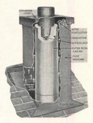
Installation time for prefabricated chimney is reported to be about two man hours
