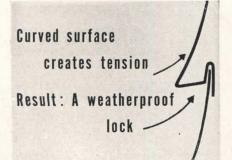
And this exclusive curved surface does even more. It is a deliberately engineered feature which makes this the strongest aluminum siding ever known. When lower edges are nailed down, the curve creates a tension which results in absolutely weathertight joints. And it creates beautiful clean lines.
