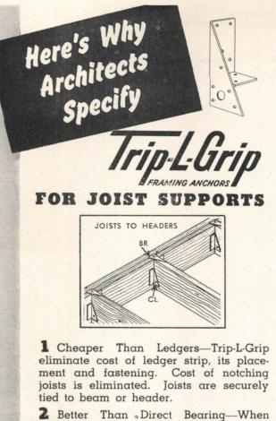
**2** Better Than Direct Bearing—When joists are placed on top of beams or girders considerable cubage is lost. Nearly 5% of the available cubage of a one-story house may be lost in this way. The cost of the extra wall height makes this expensive. Trip-L-Grip eliminate these losses.
