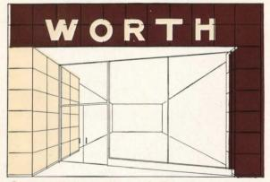
**3.** Now add the sign fascia and pilaster in a contrasting color to complete the framing. To display the store name, its product or its trade-mark, sandblast the *Vitrolite* or laminate on the fascia a contrasting color of *Vitrolite*.
