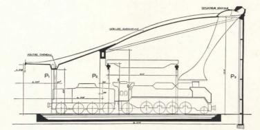
This fascinating roundhouse at Avignon, France, is remarkable for its ingenious and interesting structure, its functional architecture. The sections above show the special smokeextraction system designed to remove smoke both from the building in general and from the engines in particular. The view at the top, left, shows the extraordinary lightness of reinforced concrete construction for which French engineers are so famous
