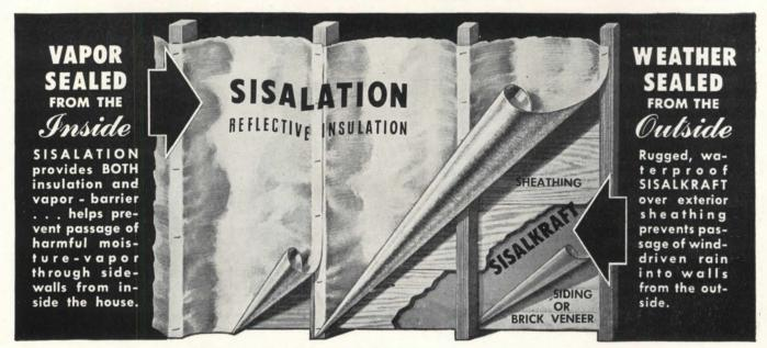
This new insulated DRY WALL construction meets FHA Vapor-Barrier Requirements (Class A, Federal Specifications UU-P-147)
