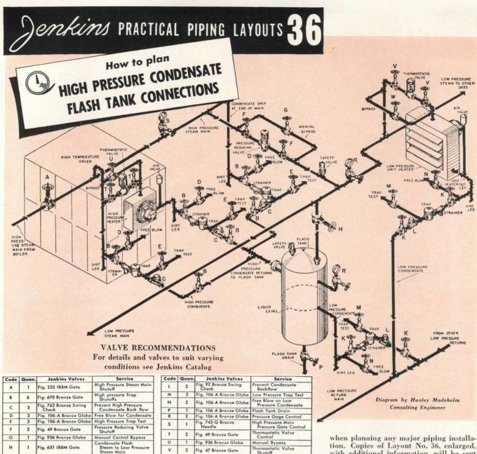
A central boiler with only one return main provides steam, in many installations, for a number of buildings spread over a wide area. To prevent disturbances caused by the flashing of the high pressure condensate discharge directly into the low pressure main, a condensate flash tank is usually installed.
