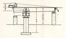
The loading operation is said to present a serious problem because (1) truck bed heights vary as much as 12 in.; (2) the truck bed moves up or down as loading or unloading progresses. The seriousness of the problem is said to have been increased with the use of power vehicles handling heavy loads.
