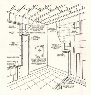
Cut-away view of x-ray room showing uses of lead for protection
