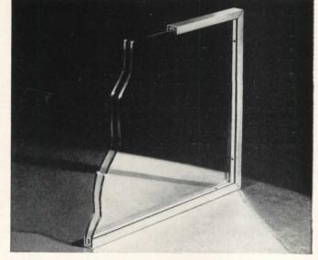
HERE'S THE SECRET of Twindow's insulating effec-tiveness. Two or more panes of Pittsburgh Glass separated by hermetically sealed air spaces. Entire unit is enclosed in a protecting frame of stainless steel.
