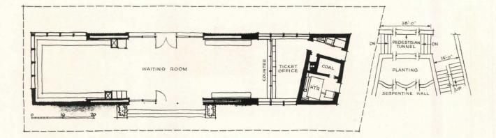
The plans are simple, and set a new standard for clean station design. An ample use of glass, which affords an almost uninterrupted vision of the platforms and train approaches from all parts of the buildings, has replaced the former unsightly bay windows common to older stations. All planning is very open, so that great crowds can pass through the station buildings rapidly without obstacles
