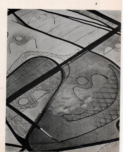
Flash firing of the glass in a gas oven at approximately 1200° makes the painted design an integral part of the glass and the window. Cooled glass is assembled (8) for final leading
