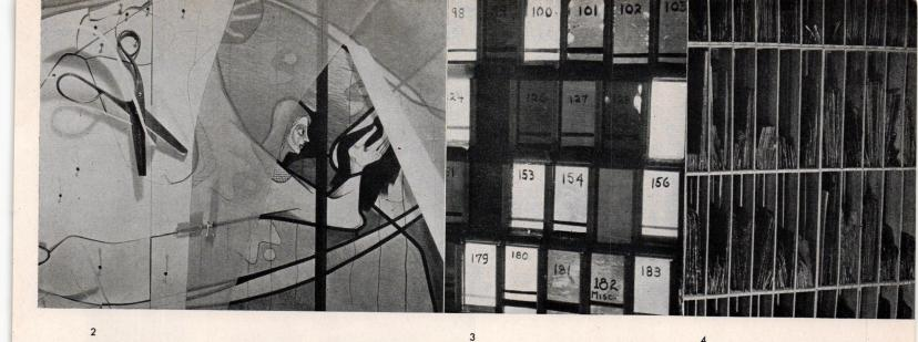
Using the cartoon as guide, patterns are cut out of paper with double-edged shears (2) which automatically allow space for the lead strips or ''cames'' between pieces of glass. Colors are matched against some 1600 numbered samples (3) keyed to compartments (4)
