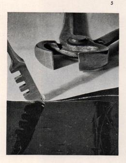
Glass is cut to the pattern with ordinary glass cutters (5) and assembled on a large piece of plate glass for viewing, after which the painted design is added (6). Colors are metallic oxides containing a flux which permits vitrification by firing
