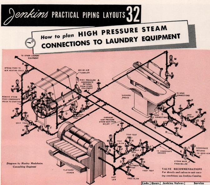
**Typical steam connections** to air drying **tumblers**, flatwork ironers, and power steam presses, commonly used in commercial or institution laundries, are illustrated in this layout.
