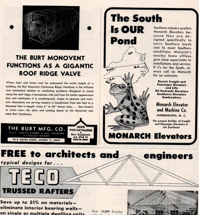
on single or multiple dwelling units By transferring the entire roof and ceiling load to the outside walls, clear span Teco Trussed Rafters eliminate the need for interior bearing walls, thus permitting complete flexibility of floor plan, both
