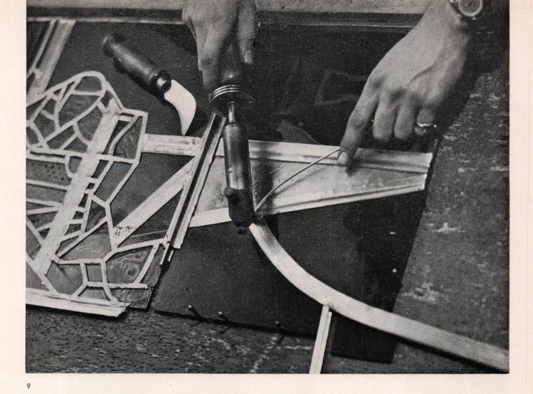
Pliable lead cames are bent, cut, placed, flattened, soldered, and a waterproof cement brushed in to hold glass securely
