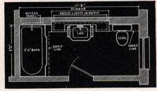
This practical, well-balanced arrangement of Kohler fixtures with all outlets leading the same way simplifies piping and allows easy access to both fixtures and storage facilities.
