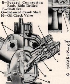
**Transverse Section through 6-Cylinder** Compressor J-Discharge Valve K-Suction-Valve Unloader L-Suction Valve M-Cylinder Liners N-Oil Check Valve -Suction Strainer 0. P-Oil-Level Sight Glass (Wide angle vision)
