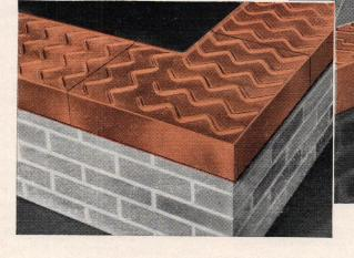
Wherever through-wall flashing is specified, as at parapets and in masonry walls, this patented Anaconda flashing offers both efficiency and durability. The design of Anaconda Through-Wall Flashing provides a complete mortar bond and prevents lateral movement in *any* direction.
