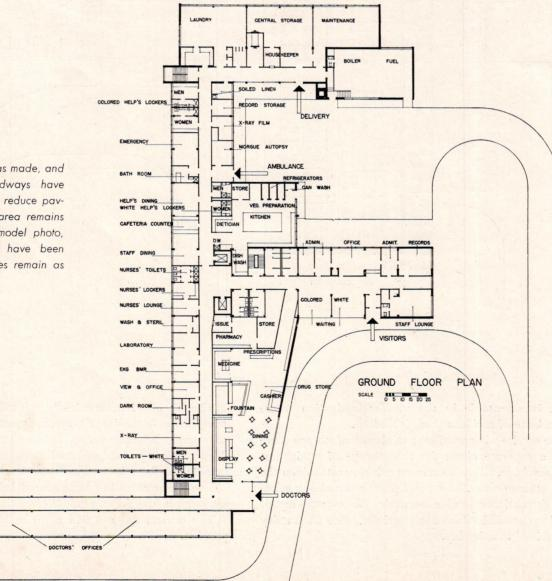
Since this model was made, and plan drawn, roadways have been replanned to reduce paving. The parking area remains as shown in the model photo, but access roads have been shortened; entrances remain as shown here
