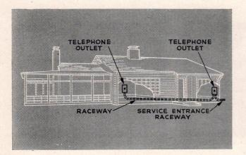
An eye to detail is important when you build livability, comfort and convenience into the small home. Telephone raceways, installed during construction, avoid exposed wires on walls and woodwork and assure greater telephone convenience to the owner.
