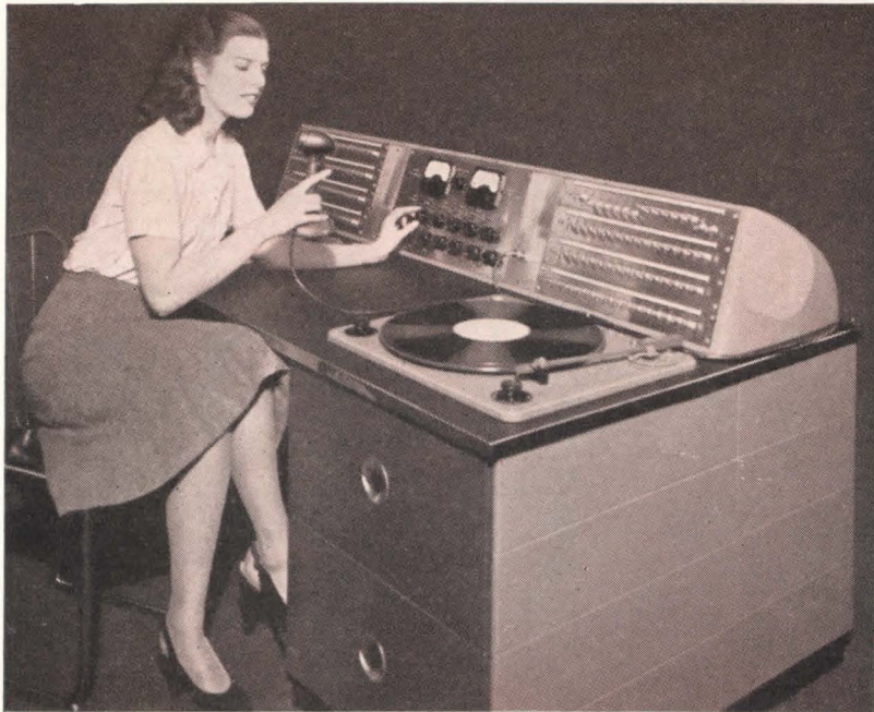
Standard frames and panels easily assemble into basic units.
