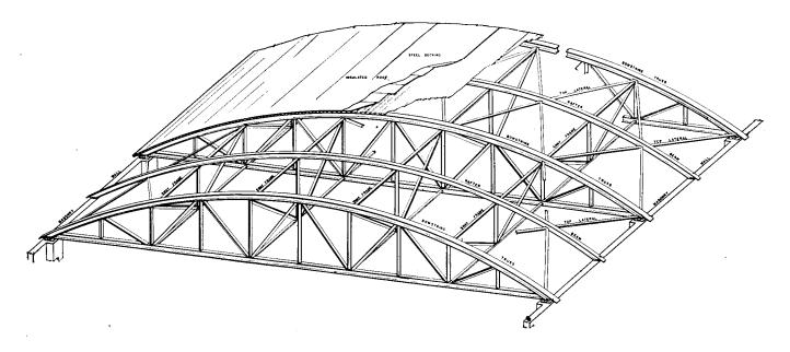
THE arc welded bow string roof truss shown above is intended for a 72-foot clear span roof supported on masonry walls, used in combination with an insulated steel deck. This type roof is ideal for large store buildings, hangars, garages, small factorics, display rooms, etc.
