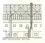
kick-up of this truss above the hangar door (see diagram) is a good idea, since the added height could be used to allow an extra opening for big tail fins if planes began to crowd the hangar in height (although it has not been so used here)
