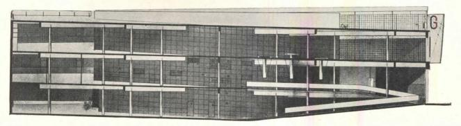
Another view of the "Spiralway" ramp parking principle applied to a G.M. dealer establishment. Low slopes permit parking on the ramp
