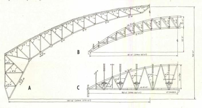
A parallel-chord steel truss structure (**D**, right) is available for large spans, cuts down height, heating, wind resistance, but consumes more material compared with the threehinged steel arch (**A**, opposite page). The small crescent wooden arch (**B**) requires either tie rods or buttresses; in the bow-string (**C**) the tie-rod is integral but the truss consumes more space
