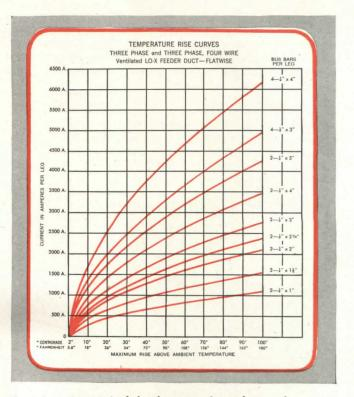
Chart shown is typical of the data on voltage drop and temperature rise available in advance of installation for all types of BullDog BUStribution DUCT. BullDog field engineers have this information at hand to help you in planning electrical distribution systems. Call the one nearest you today.
