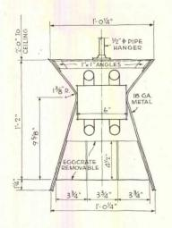
Lighting in the conference room, though very special, does not provide the wide range of combinations and control given elsewhere, since the needs are different. Fluorescent is used exclusively here, with four 2-tube open-end industrial units over the egg crate. The lowest part of the special fixture is 3 ft. 2<sup>3</sup>/<sub>4</sub> in. above the desk, to bring light exactly to the 4- by 8-ft. edges
