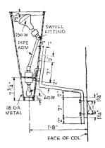
"Megaphone" fixtures above desks give glareless uniformity from the bottom over salesmen's working surfaces; from the top, provide supplement to lighting of main sales area. They are adjustable so that, to a degree, they may be thrown into incandescent-fluorescent combinations as needed. Background display screen is similar to that behind reception desk (see p. 89)
