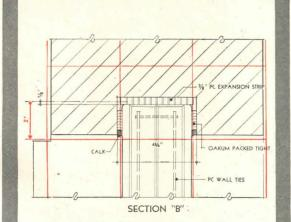
This typical jamb section illustrates the application of modular coordination to the basic principles of glass block installation. Here—and in the various modular details shown in our book—the red lines represent the standard grid based on the 4" module.
