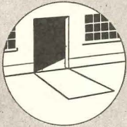
Levelator lowered becomes part of floor and can be trucked over. When loaded, Levelator rises smoothly to required level.
