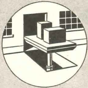
Levelator lowered becomes part of floor and can be trucked over. When loaded, Levelator rises smoothly to required level.
