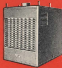
Suspended Type with Blower. Used where it is necessary to deliver air at higher velocities than possible with the propeller type fan. Models range in size from 75,000 to 450,000 Btu per hour input.
