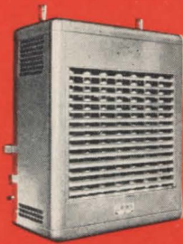
Suspended Type. The unit is suspended overhead. Propeller fan directs warm air down to the area where heat is most useful. Units range from 50,000 to 225,000 Btu input per hour.
