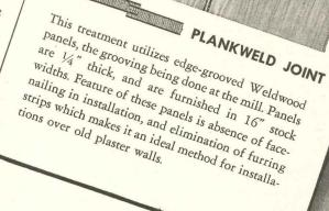
Waterproof Weldwood for exterior use is bonded with phenol formaldehyde synthetic resin. Other types of water-resistant Weldwood for interior applications are manufactured with extended urea resins and other approved bonding agents.
