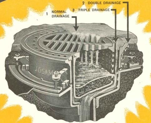
Exclusive "three-way" performance not only assures continuous, uninterrupted floor drainage in spite of accumulated debris, but also positive protection against leakage. Sediment container intercepts debris, allowing clear water to flow into drain line (normal drainage). If water seeps into floor around drain, it is returned directly into drain line...does not spread into floor or walls (double drainage). Even if sediment container becomes
