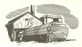
For most effective wood preservation, the chemicals must be forced deep into the wood. American Lumber & Treating Company obtain this deep penetration by the vacuum-pressure method in closed steel cylinders. Dipping, brushing on, or other makeshift methods can't begin to give comparable results. So, when you buy treated lumber, remember to say, "pressure-treated"...it's best!
