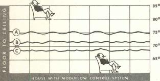
—Temperature at ceiling, B—at five foot level, C—temperature at floor
