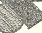
Construction of standard ¼-in. ORCO Safety Tread shown at left. Uniformly distributed abrasive grain (in nosings) and abrasive agregate (in flat surface of tread) "locked" permanently in semiresilient rubber base reresilient rubber base reinforced with 1/4-in. galvanized wire mesh.
