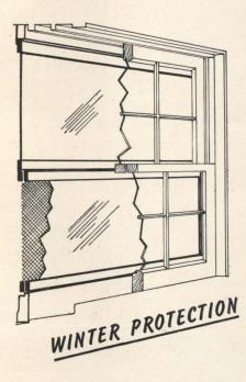
In winter, perfect window insulation is attained instantly by merely lowering Rusco storm sash. Reduces heat loss and infiltration by more than 50%-Rusco permanently insulates and weatherproofs entire window opening. Only this modern, <u>self-storing</u> window insulation gives your clients these year-around advantages !
