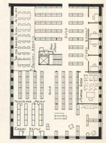
A plan study showing adaptability of Snead Bookstacks. Structural stack columns are on 12 ft. by 18 ft. centers, and all shelving, study carrels, sem-inar room partitions, etc., can be removed or rearranged quickly and easily. This permits the stack area to be used interchangaably for book storage, staff work or readers, and makes the stack adaptable to meet the ever-changing demands of a library. Study and seminar rooms are enclosed by Snead Steel Mobilwalls.
