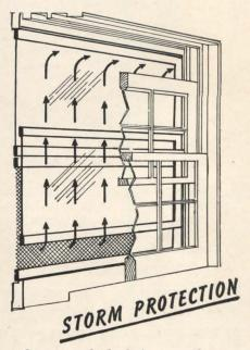
Stormproof, draft-free ventilation winter or summer by raising lower Rusco sash part way, lowering upper inside sash. Air deflects upward into room – permits open window ventilation with complete safety from storm damage or drafts.
