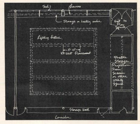
Fixture pattern is seen in plan, above. As drawn, it uses 28 100-watt F lamps, with auxiliaries, the output becomes 117,600 lumens.
