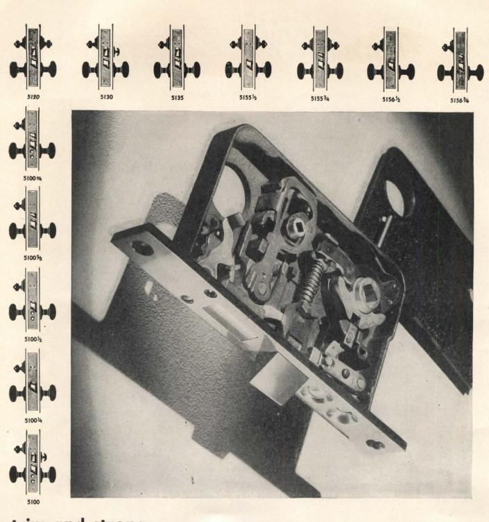
trim and strong . . . this Lockwood Cylinder Mortise Lock is one of a long line providing 26 different locking functions, standardized as to size, backset and spacing. Some of them are shown bordering the above picture. Every lock fits into the same mortise. Essential parts are of forged bronze for extra strength, smoother operation. Knob action is semi-poised for greater turning ease in either direction.
