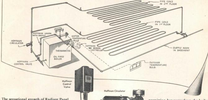
The sensational growth of Radiant Panel Heating has made necessary the development of special equipment to best serve its unusual characteristics. Designed with these requirements in mind, the Hoffman 90 Series System precisely controls and maintains the relatively low temperature required by radiant panels. It has proved
