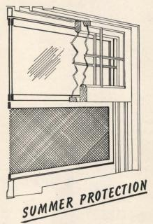
In summer, Rusco storm sash simply slides up into storage position, giving full, direct ventilation through permanent Rusco screen.
