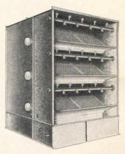
**CAPILLARY AIR WASHERS** are available in a series of five height sizes, and in eleven widths — capacities from 4,400 to 132,000 c.f.m. They are built in Class I (con-current), Class II (counter-current) and Class III (concurrent with coils) types. Bulletin 120 describes complete line of equipment.
