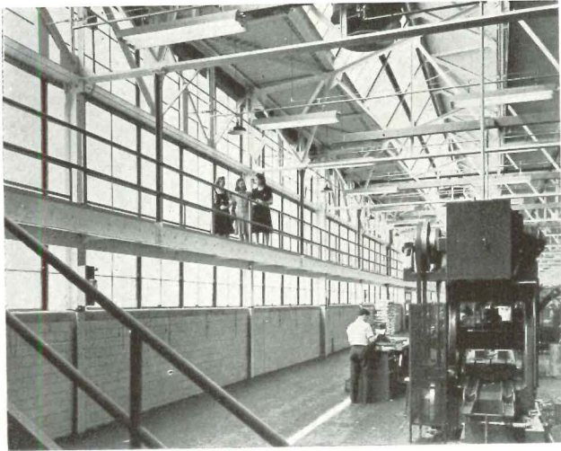
Pedestrian walkway off the production floor. "It was found desirable to add a shield along the inner side to prevent swirling skirts above from offering too much distraction"
