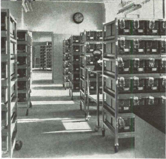
Movable animal cages are in gray-tiled, cove-based, sanitary rooms, with floor of beige terrazzo. Floor drains are provided. Air conditioning is a separate system, with temperature and humidity control for each room. Outdoor animal cages have remote-control sliding doors to inside portions
