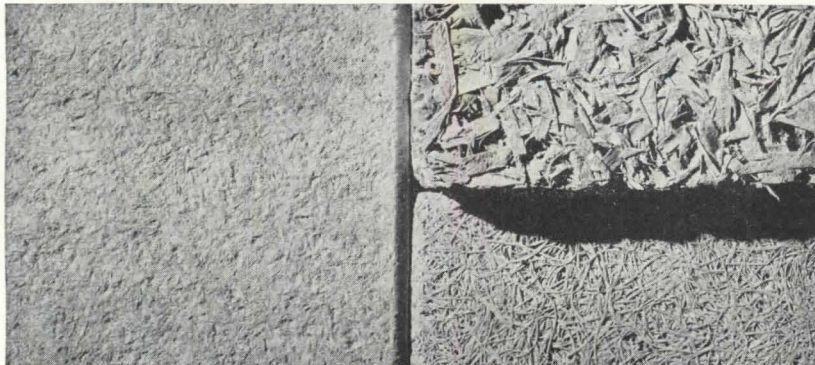
Left: Fibercoustic, federal specification number VIII; upper right: Absorb-A-Noise tile, VII; lower right: Absorb-A-Tone VII
