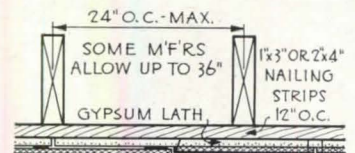
PREFERRED METHOD - NEW WORK. BOTTOMS OF JOISTS NEED NOT BE LEVEL ON WOOD FURRING STRIPS AND GYPSUM LATH
