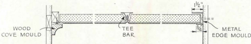
NOTE - WOOD MOULDS & WORK ABOVE TEE BAR NOT USUALLY INCLUDED IN ACOUSTICAL SPECIFICATIONS
