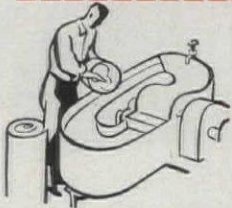
Plastic in form of resin is added to a mixture of paper pulp and water in a beater of type used in paper mills.
