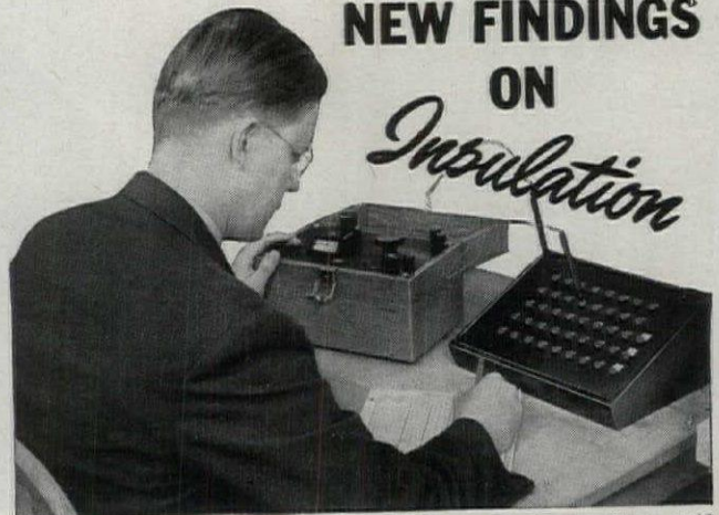
Taking temperature readings at 43 thermocouples with potentiometer.
