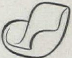
When air is evacuated from die, vacuum attracts pulp particles, producing preform approximate shape of chair.
