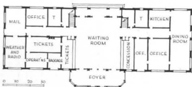
Basic floor plan requirements for an inexpensive administration building for a small airport, as suggested by CAA
