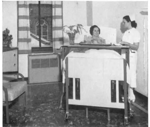
NO DRAFT — NO DUST — NO DIN. Windows are always closed and the temperature in private patients' rooms in the new wing is always the best for rapid recovery, thanks to the new air conditioning conduit system which permits individual control in each room.
