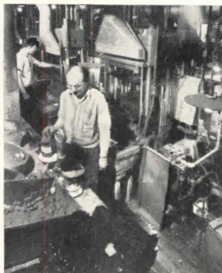
Hydraulic Pressing of panel units and large circuit breakers. A single panel unit requires application of 100 tons pressure, using combination of powder and pre-forms.
