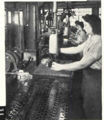
At right: Drilling circuit breakers. Holes of small diameter may be drilled more economically than molded under the pressing operation.
