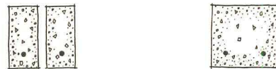
Pre-cast concrete lintels, requiring steel only in the pencil rod reinforcing, may be used in place of steel lintels, with considerable metal saving
