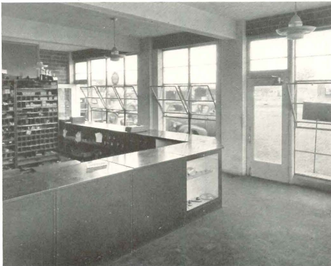
OFFICE: glazed walls facilitate supervision of yard
